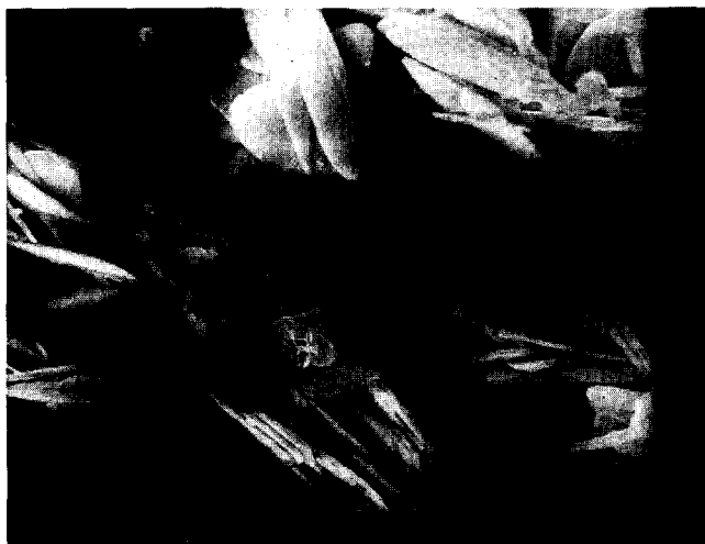
FIG. 1. Scanning electron micrograph of precipitated tungstic acid, \text{H}_2\text{WO}_4, \text{H}_2\text{O} (JCPDF 18-420).
